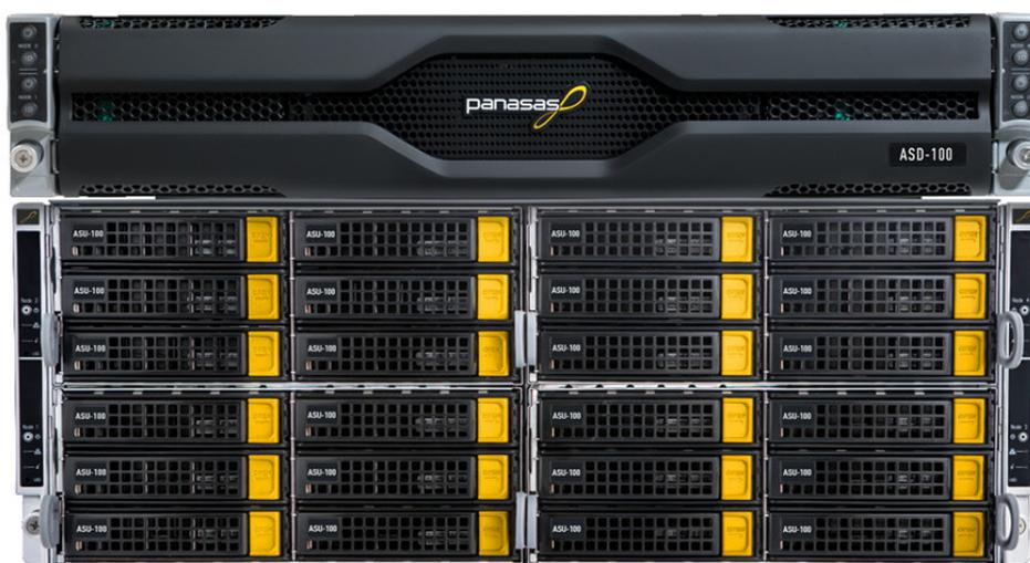
Panasas “ActiveStor” is a clustered scale-out NAS appliance designed for speed and reliability.
